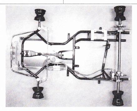
PHOTO FROM ABOVE OF COMPLETE CHASSIS IDENTICAL TO ONE OF THE MODELS SUBMITTED FOR REGISTRATION WITHOUT BUMPERS, BODYWORK, OR TYRES
