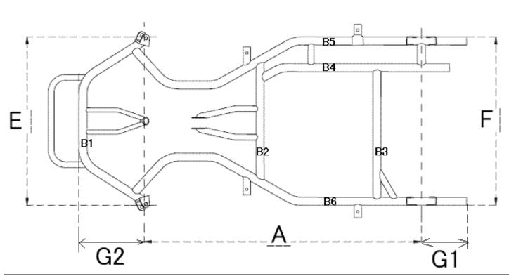
Only show tubes from the structure and fixations sustaining the stub axles and the stiffening bars that require details and dimensions as featured in section B
